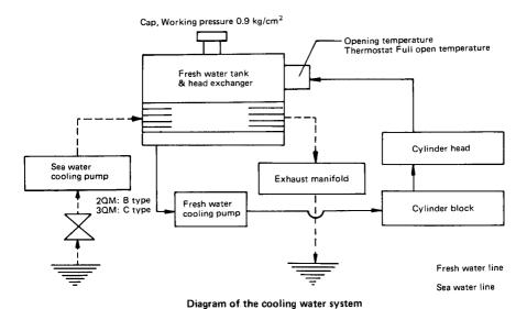
Cooling Water Pump (Fresh Water) & Heat Exchanger
