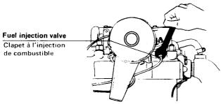
5) Set the speed control lever to the FULL position.
